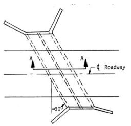
Measurement for a skewed box under fill.
