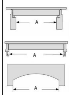
Figure 15. Profile views of various single span bridges.
