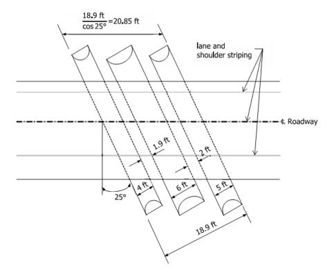
Multiple pipes may be considered a bridge if the distance between the pipes is less than half of the smallest opening and the structure length is greater than 20 feet. In the above illustration, the structure length is recorded as 20.85 feet.
